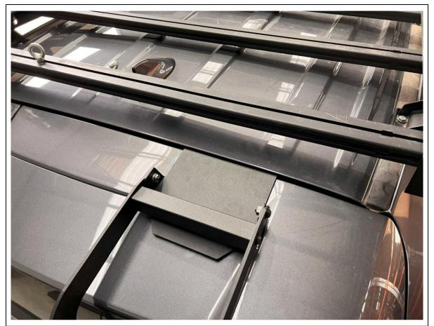
13. Lift the ladder up to the Ladder top plate and secure with M8 x 20 Button Head Cap screws, washers, and flange nuts.
