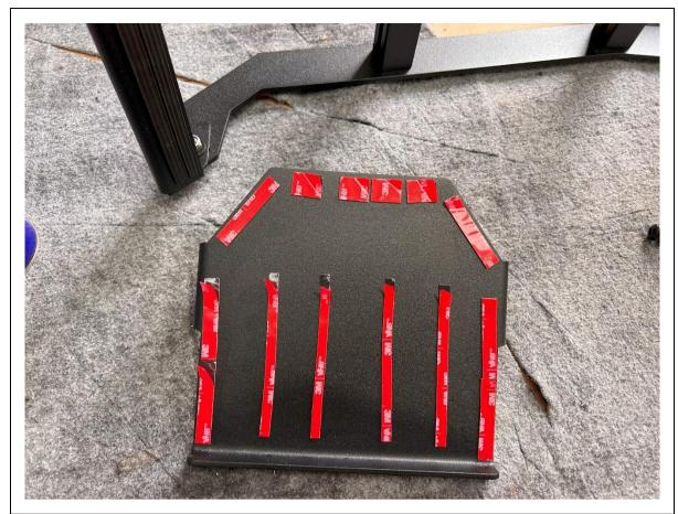
9. Apply double sided tape to the Ladder top plate as shown.
