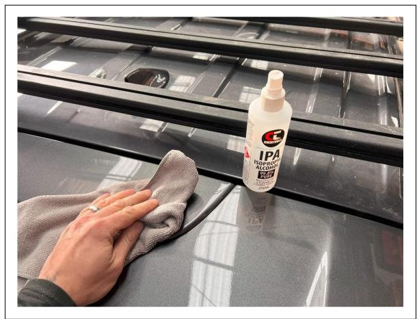
5. Climb up on the rear bumper or suitable step ladder to show the top of the rear tailgate and thoroughly clean the whole area with Isopropyl alcohol.
