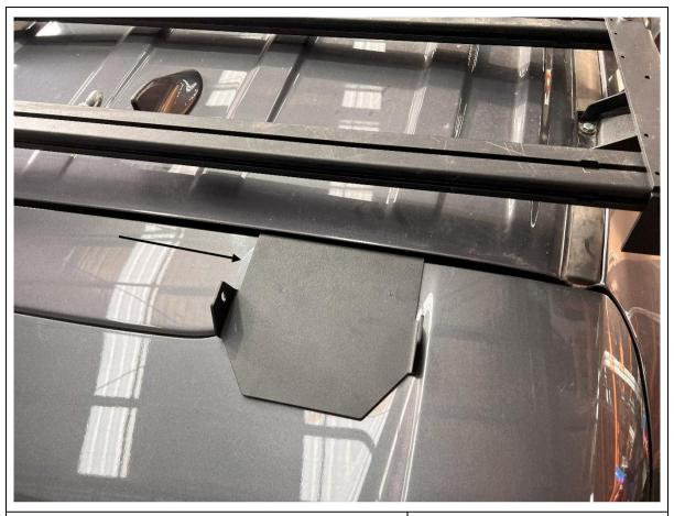
10. Remove tape backing and Stick Ladder top plate to the top of the tailgate as shown.
